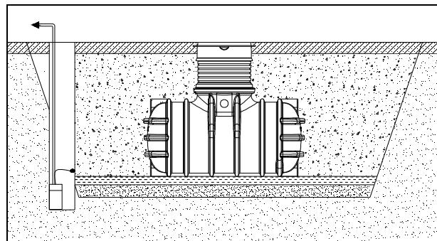
The pump should be checked regularly. The size of the pipe depends on the size of submersible pump used. The float switch must be able to function fully at all times.
