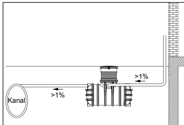
**Important:** The empty pipe should be connected to an opening **above** the max. water level.
