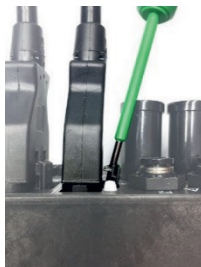
Figure 16: Loosening the claw for the 230 V plug
