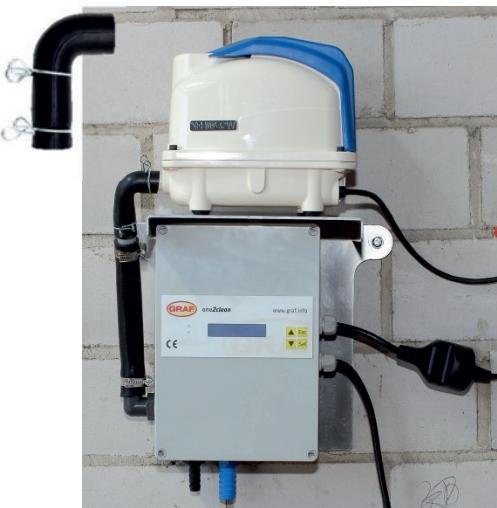
Position the compressor on the control. Connect the compressor to the control unit pipe using the 90 deg. hose piece and hose clamps provided. Plug the compressor plug into the control socket.
