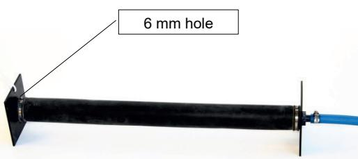
The cord must be secured to the membrane tube aerator(s) (6 mm hole). The air hose (19 mm) must be connected on the opposite side. Systems for more than 7 inhabitants have two membrane tube aerators.
